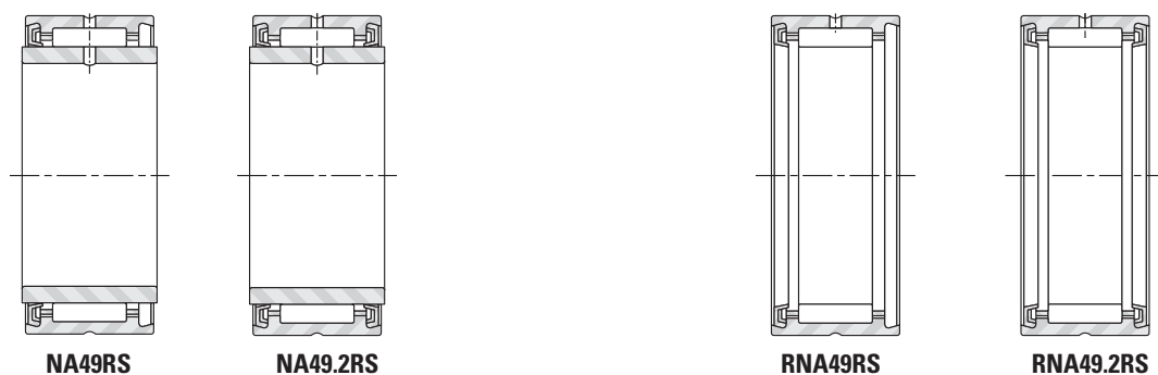
Fig. B4-3. Sealed needle roller bearings with inner rings
